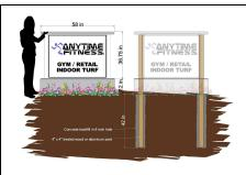
1. Dig two holes in ground (spacing is determined by existing holes in the monument base cap). Mount two 4x4 treated wood posts in the holes using concrete.
